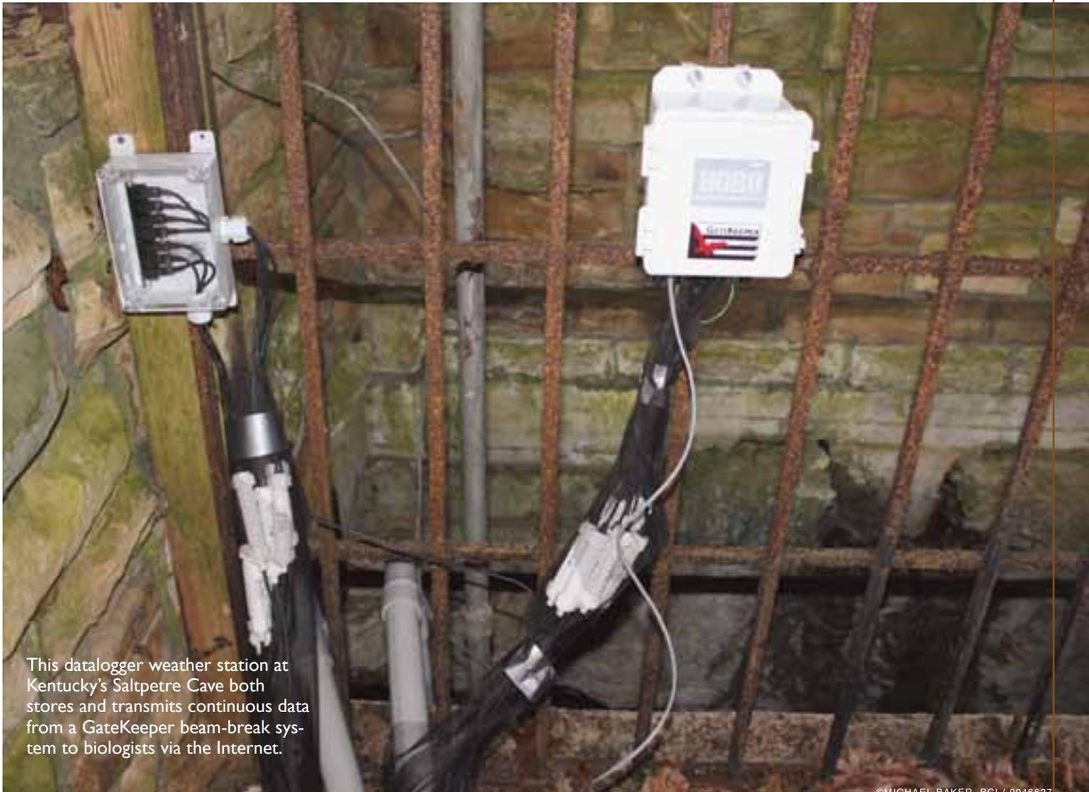
This datalogger weather station at Kentucky's Saltpetre Cave both stores and transmits continuous data from a GateKeeper beam-break system to biologists via the Internet.
